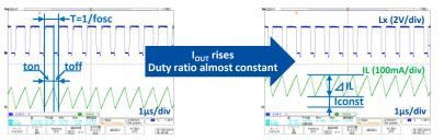
• Ideal Duty ratio and ton of step-down DC/DC at CCM PWM operation are ton = (1/fosc) x Duty = (1/fosc) x  $(V_{OUT}/V_{IN})$ . If there is no loss, **Duty ratio is constant** even if I<sub>OUT</sub> rises.
