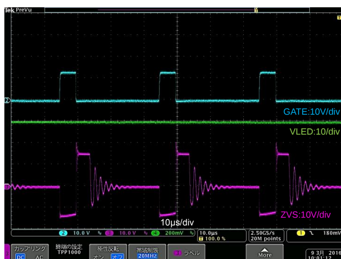
Fig. 4: Transformer auxiliary voltage and ZVS pin voltage
