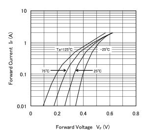
(3) Forward Voltage vs. Operating Temperature
