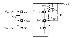
Example of external components (V<sub>OUT</sub>=1.8V)
