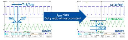
Ideal Duty ratio and ton of step-down DC/DC at CCM PWM operation are ton = (1/fosc) x Duty = (1/fosc) x (V<sub>OUT</sub> / V<sub>IN</sub>).
